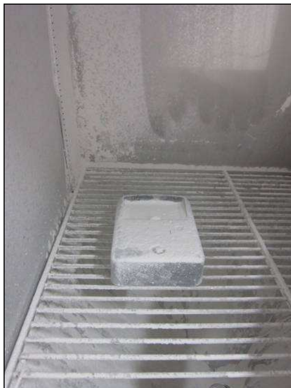
Fig. 4 Samples in the chamber after dust test
