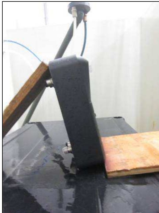
Fig. 8 Positioning of the sample inside the salt mist chamber
