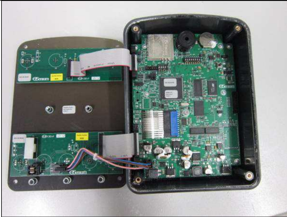
Fig. 5 Samples during the visual inspection after dust test
