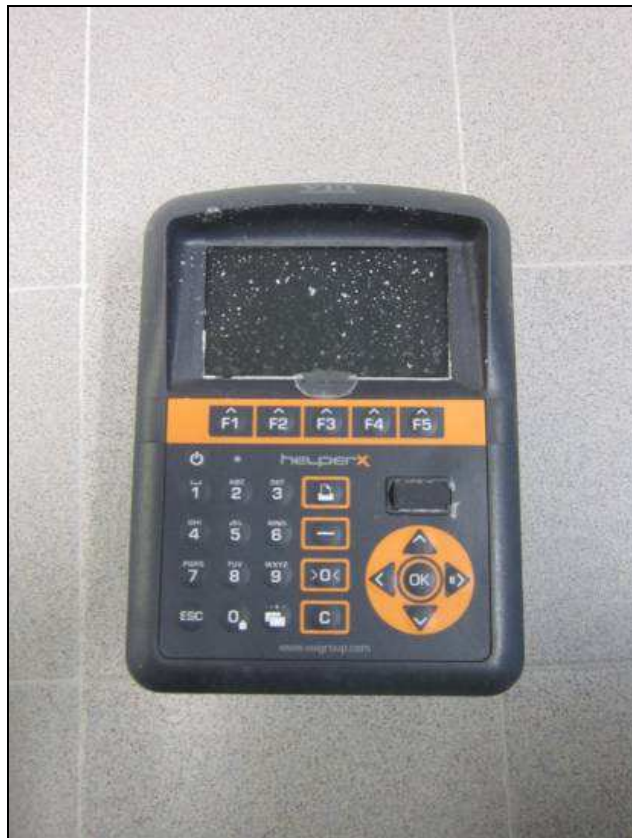
Fig. 9 Sample after salt mist test
