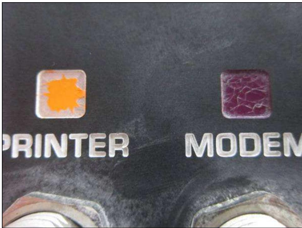
Fig. 7 Coloured labels after the climatic test
