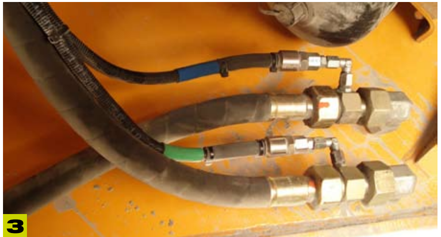
Load sensors installed on the hydraulic circuit of the lifting arms. One sensor is installed on the main pressure side of the lifting cylinder, while the second sensor is installed on the anular side.
