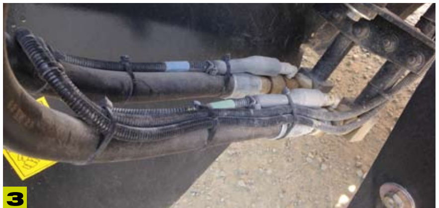
Load sensors installed on the hydraulic circuit of the lifting arms. One sensor is installed on the main pressure side of the lifting cylinder, while the second sensor is installed on the anular side.
