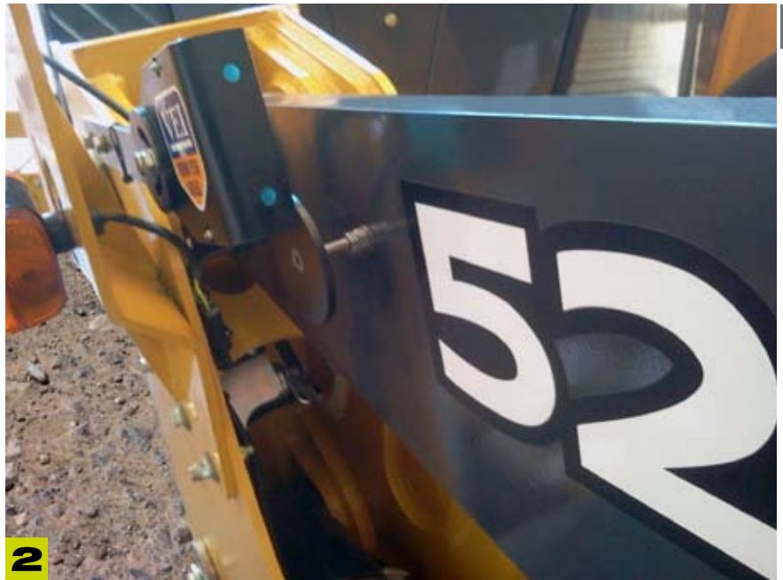
Contactless weighing zone sensor for weight reading.
