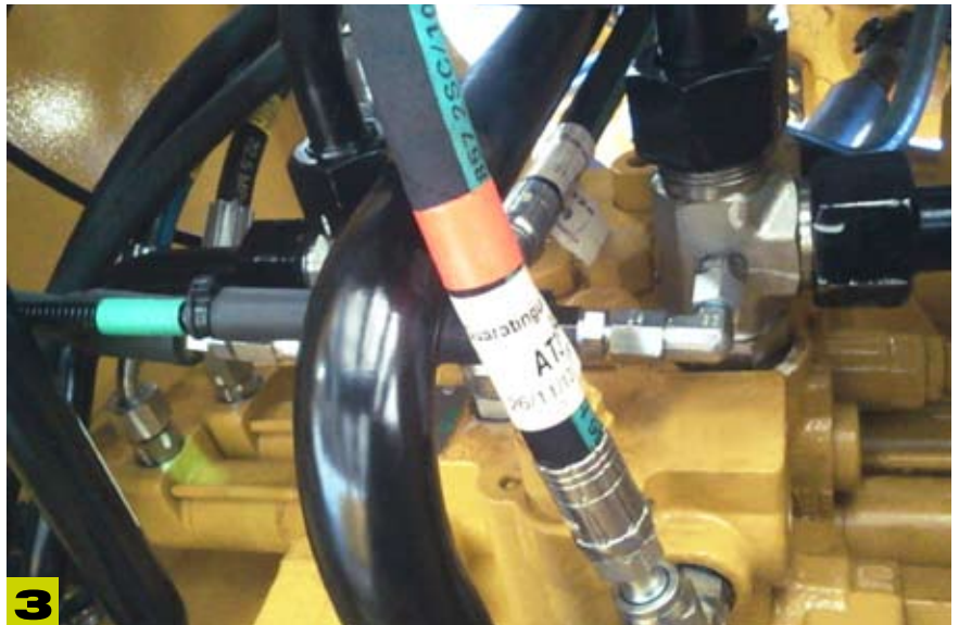
Load sensors installed on the hydraulic circuit of the lifting arms. One sensor is installed on the main pressure side of the lifting cylinder, while the second sensor is installed on the anular side.
